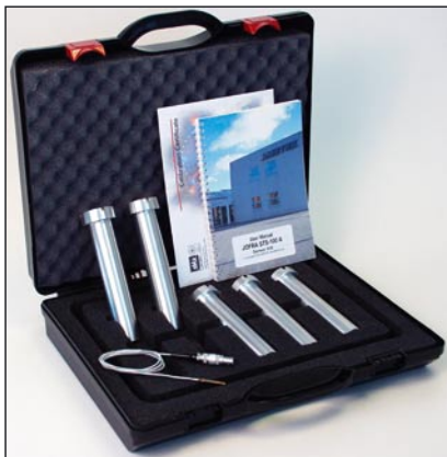
A complete application kit for calibration of sanitary temperature sensors with »clamp«.
