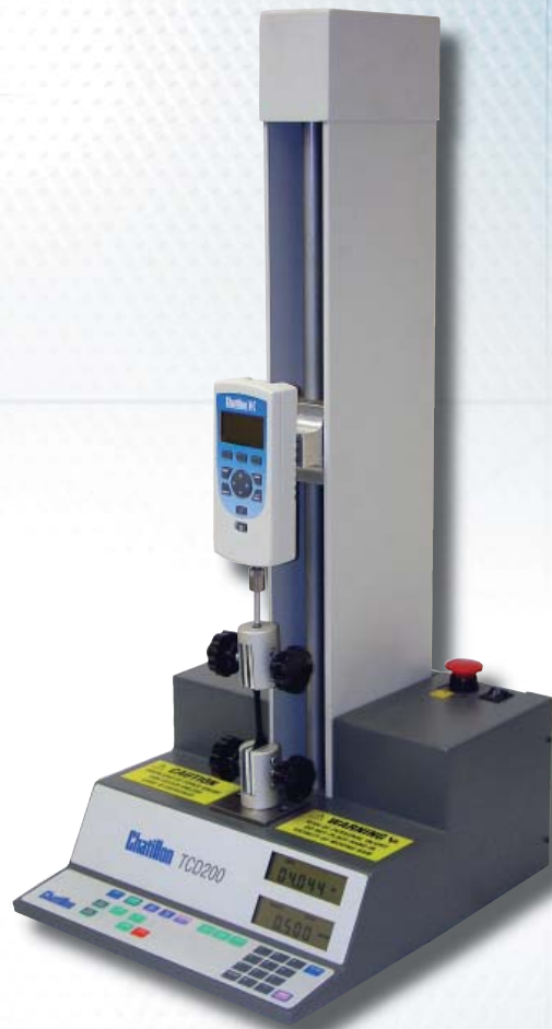
TCD200 with DFS Series digital force gauge
